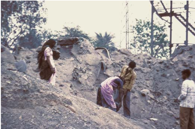
Fig. 2.10 Unprotected young female workers recycling lead oxide in an Indian lead refinery; a dramatic example of what not to do.
