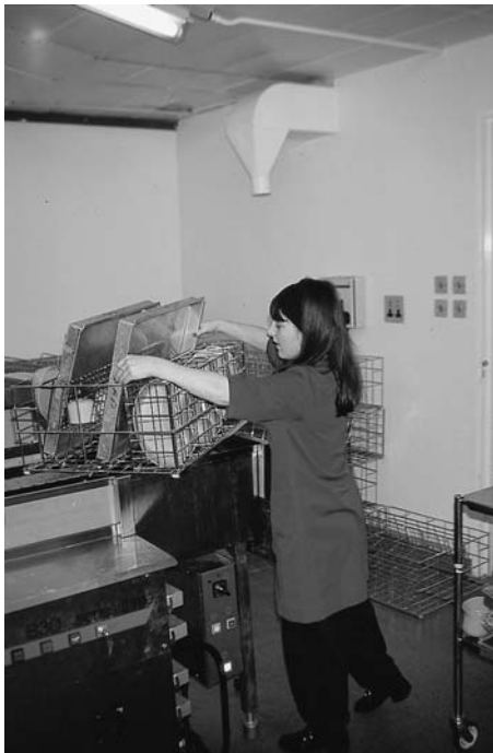
Fig. 5.4 Bad ergonomics. A short operator in a hospital sterilizing department having to fill and empty trays on a washing machine at the extreme limit of her reach. See also colour plate 5.4.
