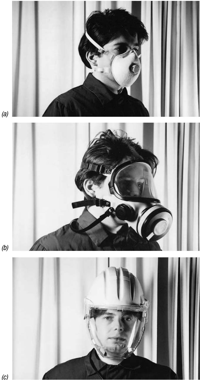
Fig. 6.2 (a) Filtering facepiece respirator to provide a moderate level of protection against dusts and other aerosols. (b) Full-face powered respirator which will provide a high degree of protection against dusts and other aerosols. (c) Powered helmet respirator. Air is drawn from behind the head, filtered to remove any particles and blown over the face. The unit also provides head protection and a visor to protect the face. (continued)
