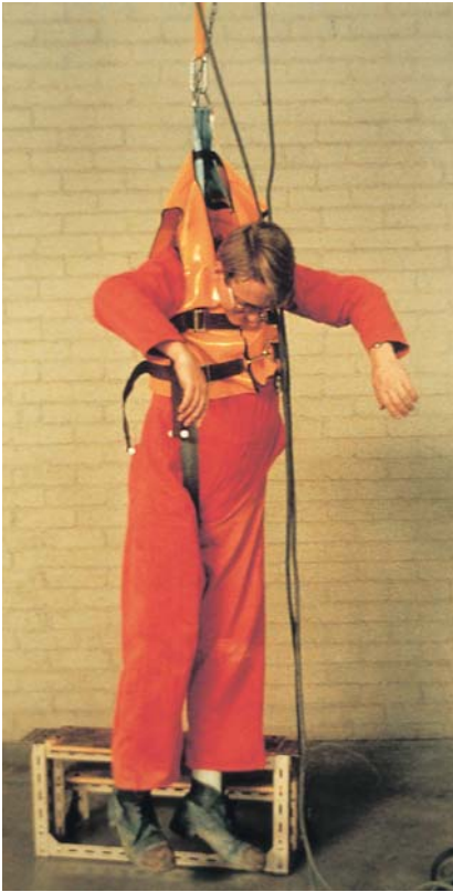
Fig. 5.1 Consequence of inadequate design of safety harness and training in its use.
