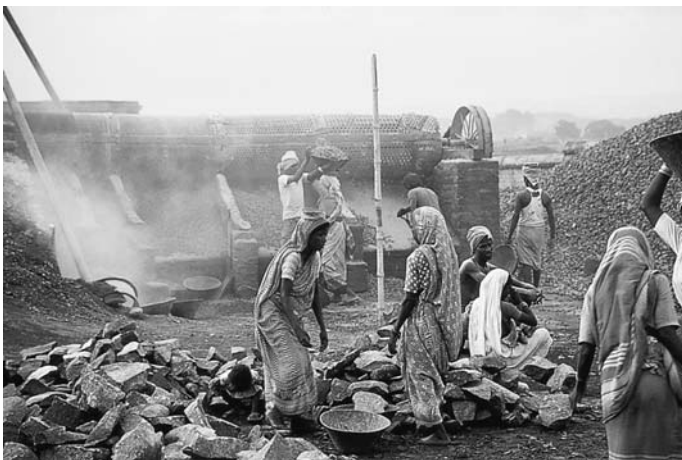
Fig. 7.1 Women and children working at a roadside stone-crushing plant in rural Bihar, India. High, lifelong dust exposures are inevitable. See also colour plate 7.1.
