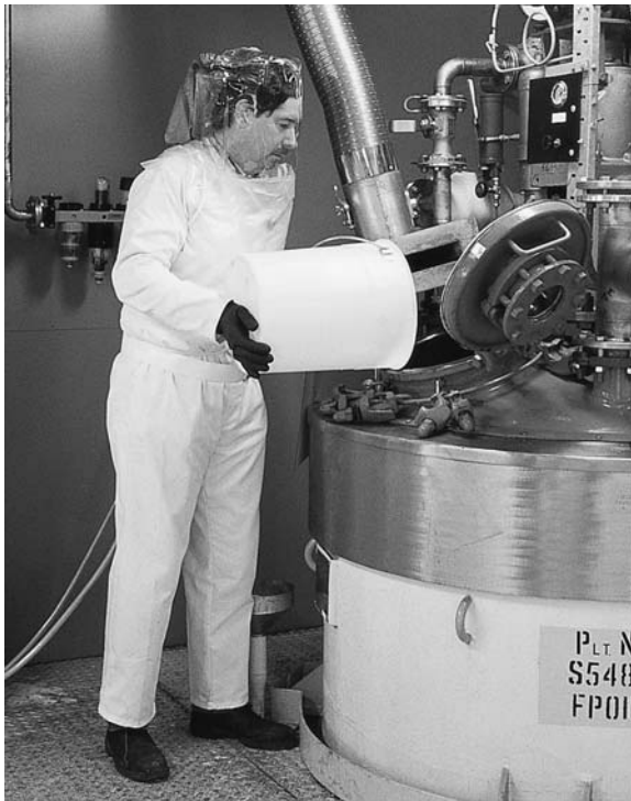
Fig. 6.2 (d) Ventilated suit used to provide higher level of respiratory and body protection against radioactive dust. (e) Personal protection including breathing air being delivered through an air hood in the chemical industry. Note also local exhaust ventilation through a flange overlying the reaction vessel next to the potential emission source. (Photographs courtesy of Dr John Cherrie.) See also colour plates 6.2(d) and (e). (continued)
