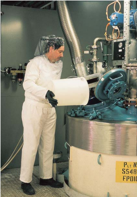
Fig. 6.2 (e) Personal protection including breathing air being delivered through an air hood in the chemical industry. Note also local exhaust ventilation through a flange overlying the reaction vessel next to the potential emission source. (Photographs courtesy of Dr John Cherie.)
