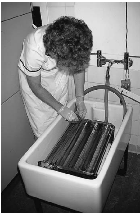
Fig. 3.6 Washing a unit from the X-ray processor. Normally this is enclosed but has to be removed on a regular basis for cleaning, allowing exposure to chemical vapours. See also colour plate 3.6.
