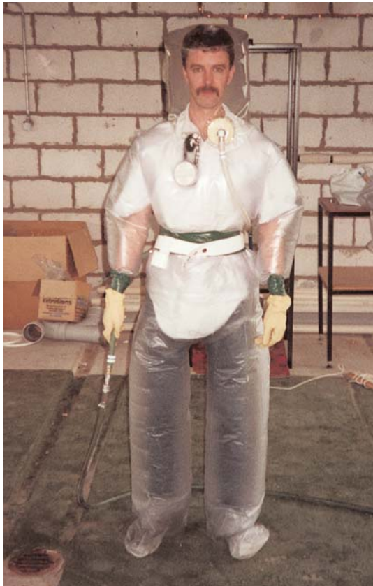
Fig. 6.2 (d) Ventilated suit used to provide higher level of respiratory and body protection against radioactive dust.
