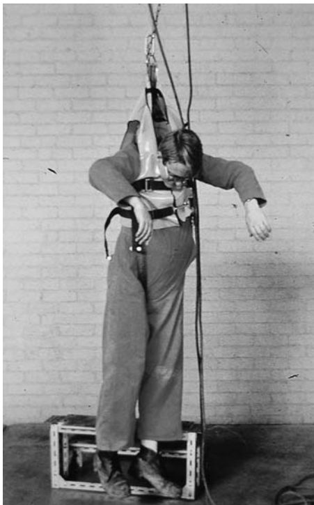
Fig. 5.1 Consequence of inadequate design of safety harness and training in its use. See also colour plate 5.1.
