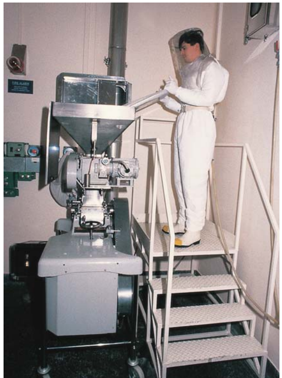
Fig. 6.2 (e) Personal protection including breathing air being delivered through an air hood in the chemical industry. Note also local exhaust ventilation through a flange overlying the reaction vessel next to the potential emission source. (Photographs courtesy of Dr John Cherie.)
