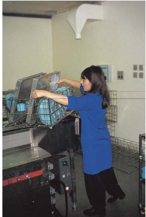
Fig. 5.4 Bad ergonomics. A short operator in a hospital sterilizing department having to fill and empty trays on a washing machine at the extreme limit of her reach.
