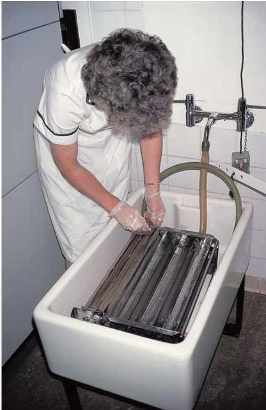
Fig. 3.6 Washing a unit from the X-ray processor. Normally this is enclosed but has to be removed on a regular basis for cleaning, allowing exposure to chemical vapours.
