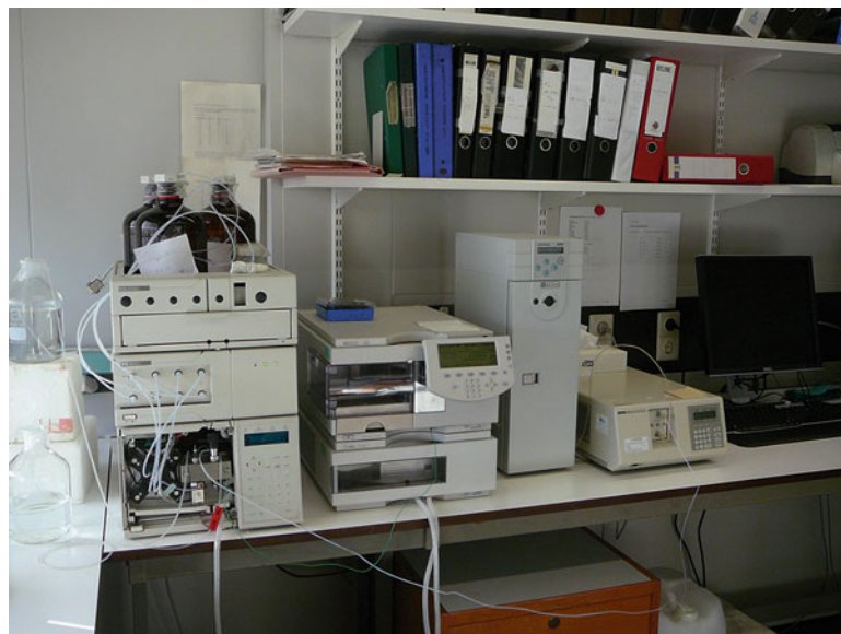
Fig. 1. Equipment used for the HPLC analysis. Left apparatus from top to bottom : Solvent cabinet, degasser, and quaternary pump. Second apparatus : Autosampler with control module and cooling unit. Third apparatus : Column oven with Peltier cooling device. Fourth apparatus : Fluorescence detector. Most right apparatus : Computer for data acquisition.
