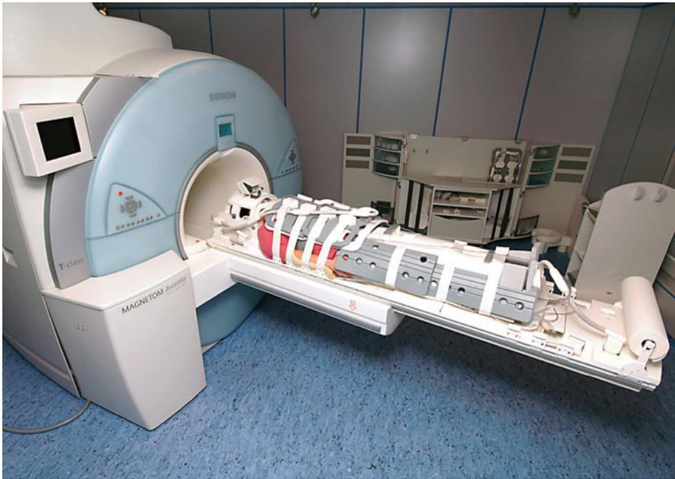
**Fig. 1.** Multiple coils optimized for each body region and comprising up to 76 elements and up to 32 receiver channels cover the whole human body. With this total imaging matrix (TIM; Siemens, Erlangen, Germany) technology a length of 2.05 m from head to toe can be scanned with sequential or continuous table movement.
